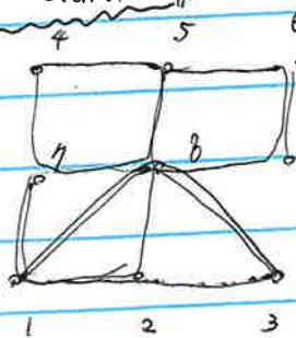
$$LV = \begin{pmatrix} 1 & 2 & 7 & 8 \\ 2 & 3 & 8 & 9 \\ 8 & 1 & 5 & 6 \\ 7 & 8 & 4 & 5 \end{pmatrix} \quad \left. \begin{array}{l} \text{Basis} \\ \text{Functions.} \end{array} \right.$$
