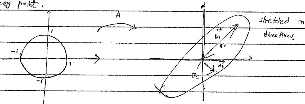
1) Left singular vectors: semi-axes of resulting ellipse.
