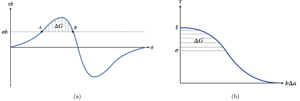
Figure 1: Stress acting on a dislocation while gliding in two different perspectives where (a) energy landscape diagram respect to the total dislocation swept area  $a$  with the activation free energy  $\Delta G$  inside the shaded region and (b) glide resistance diagram showing the stress  $\tau$  experienced by the dislocation respect to the change of the swept area (i.e., activation area)  $\Delta a$ .
