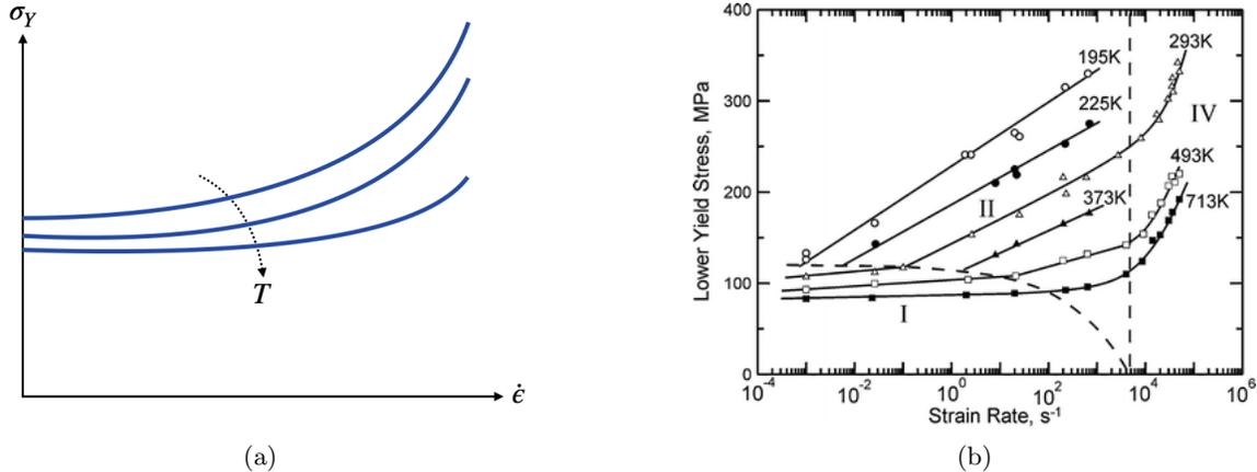
Figure 2: (a) Yield stress with respect to the strain rate predicted from the equations relating the activation rate to stress-dependent activation free energy and (b) experimental data of the yield stress with respect to the strain rate for ferritic stainless steels.
